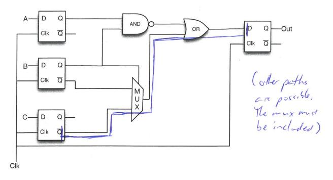
For the following subquestions, use the circuit above and assume that each 2-input boolean gate has a propagation delay of 30 ns and contamination delay of 15 ns. (NOT gates are free.) Assume that a D flip-flop has a clock-to-q propagation delay of 80 ns, setup time of 120 ns, hold time of 70 ns, and clock-to-q contamination delay of 40 ns.
