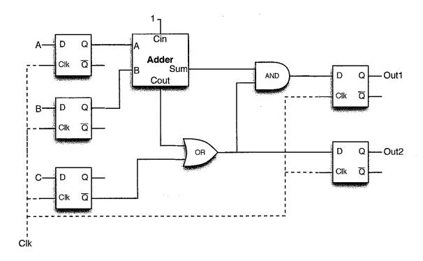
For the following subquestions, use the circuit above and assume that each 2-input boolean gate has a propagation delay of 20 ns and contamination delay of 10 ns. (NOT gates are free.) Assume that a D flip-flop has a clock-to-q propagation delay of 60 ns, setup time of 25 ns, hold time of 35 ns, and clock-to-q contamination delay of 30 ns.
