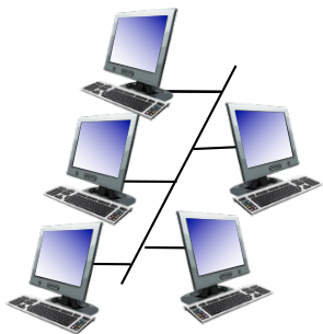
shared wire (e.g., cabled Ethernet)
