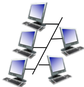
shared wire (e.g., cabled Ethernet)
