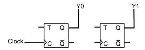
(b) Below, complete the circuit of a 2-bit **synchronous 0-to-2 counter**, i.e., upon each clock cycle, the value represented by **Y1Y0** changes like 0, 1, 2, 0, 1, 2, 0, 1, 2, 0, etc. You are ONLY allowed to add wires, constant input values (such as 1 or 0), and **at most one instance** of **AND** gate or **OR** gate, i.e., you're NOT allowed to use more than one logic gates, and you're NOT allowed to use any logic gate other than AND and OR. [4 marks]
