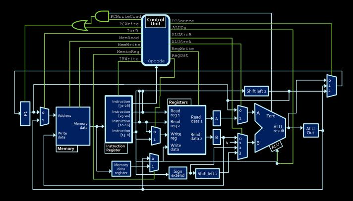
Given the datapath above, what signals would the control unit turn on and off to increment the program counter by 4?
