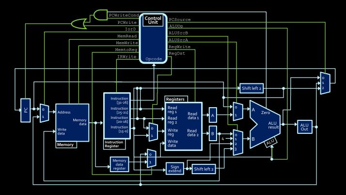
Given the datapath above, what signals would the control unit turn on and off in order to add \$r1 to \$r2 and store the result in \$r7?
